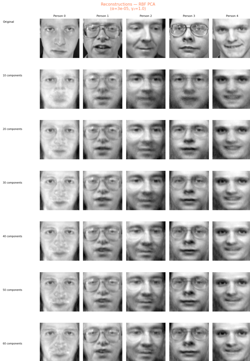
Figure 7 Row 1 shows 5 images taken from the dataset. Each successive row shows the RBF reconstruction of an image with 10, 20, 30, 40, 50 and 60 principal components respectively.
